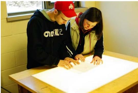
Skene house and the Sinclair additions were each crossdated with these references to determine their age. This was accomplished by matching growth-curve patterns of the references with the building. A light table (photo left) was used to help visually compare our ring growth graphs by observing recognizable patterns in the tree-ring sequences
