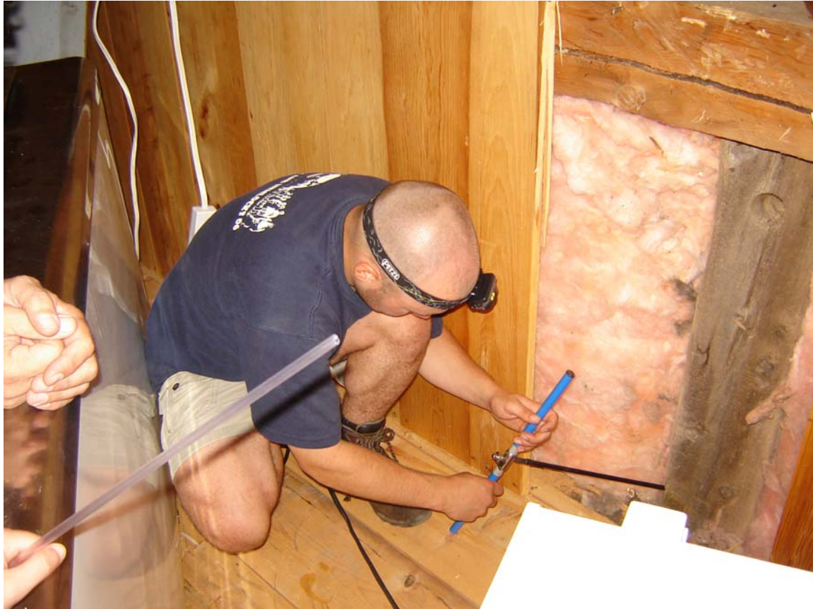
Figure 2: Openings in the paneling were created to gain access to ten main upright beams. A researcher is shown using an increment boring tool to collect a 4.3 mm sized dowel from the beam.
