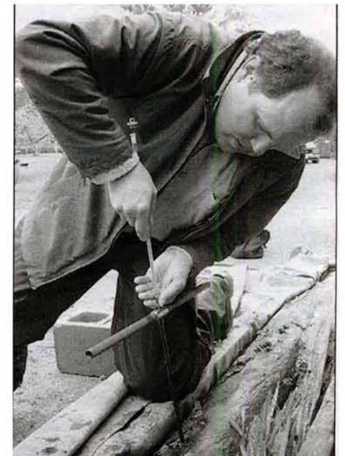
Mount Allison dendrochronologist André Robichaud takes a core sample from the spruce log found next to the sluice.
