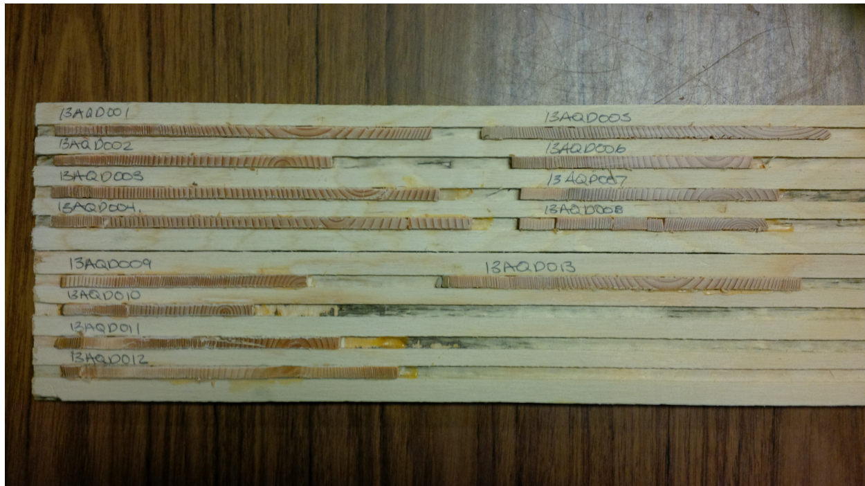
Figure 1: Core samples taken from the “Dickson House” structures. Cores were glued to a slotted mounting board and were sanded with progressively finer sand paper. Annual-growth rings are clearly visible after sanding.
